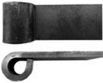
HINGESTRAP5123080 5mm thick, 12mm hole, 30mm wide, 80mm length
