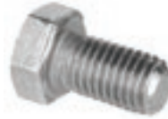
BIF38X1-5Z \frac{3}{8} -inch UNF bolt 1-inch long grade 5 zinc
