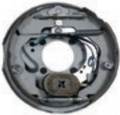
EB12LPG 12-inch galvanised backing plate - left
