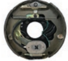
EB12RP 12-inch black backing plate - right
