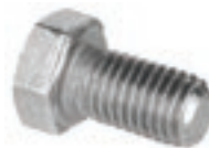
BIF716X1-5Z 7/16-inch UNF bolt 1-inch long grade 5 zinc
