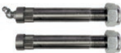
SASBSS16100 – Non-greaseable SAGBSS16100 – Greaseable ⅝-inch (15.8mm) bolt 304 stainless suits 60mm spring
